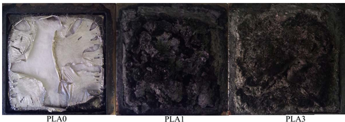
Figure 8. Digital photographs of the char residue after the cone calorimeter test. [Color figure can be viewed in the online issue, which is available at wileyonlinelibrary.com .]
